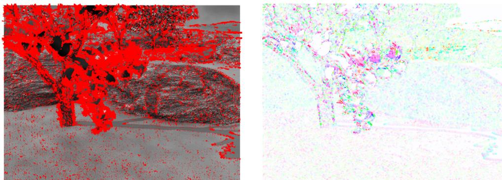
Figure 4.22: Optical flow field estimated by Lucas and Kanade for Grove2 example.
